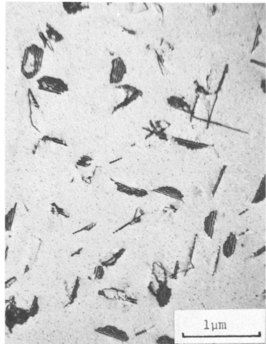
Figure 2 Co-25 Cr-10 Ni-0.25 C alloy, solution treated 1 h at 1300°C, water quenched and aged 2 h at 700°C. Bright-field micrograph showing the matrix precipitates and stacking faults.
